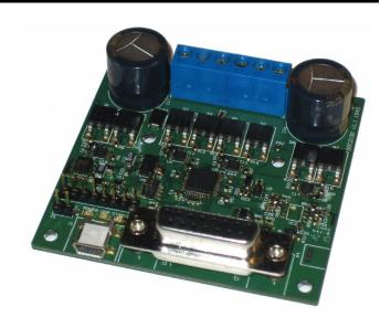
Fitting a very compact 70x70mm board, Roboteq's SDC21xx controller is designed to convert commands received from an RC radio, Analog Joystick, wireless modem, PC (via RS232 or USB) or microcomputer into high voltage and high current output for driving one or two DC motors. A version with CAN bus allows up to 127 controllers to communicate at up to 1Mbit/s on a single twisted pair.
