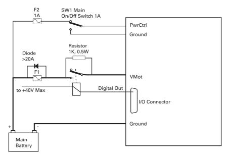
FIGURE 10. Contactor wiring diagram
