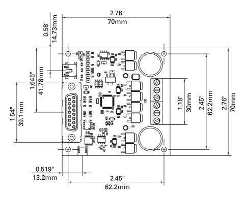
FIGURE 17. SDC21xx top view and dimensions
