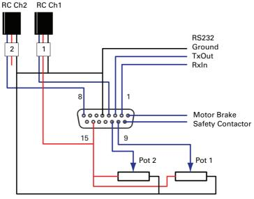
FIGURE 13. Factory default pins assignment
