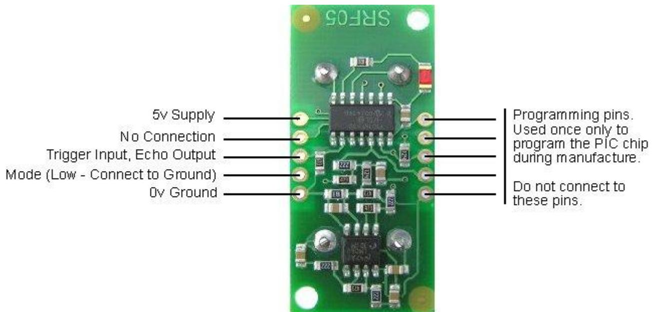
Connections for single pin Trigger/Echo Mode
