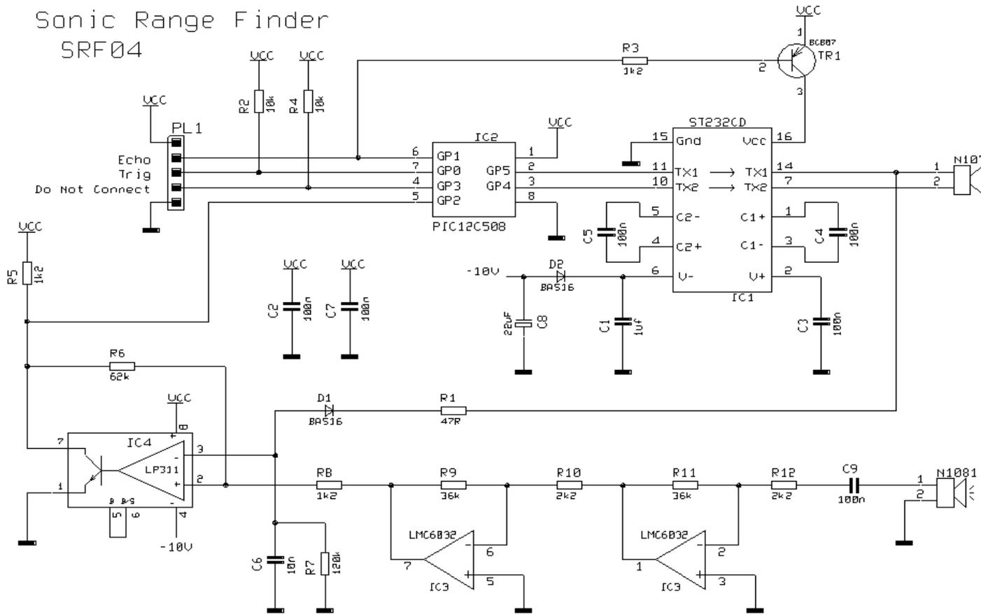
LMC6032 Pin 4 Connected to -10v
